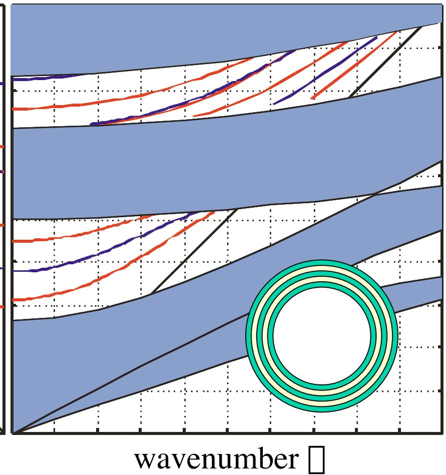
modes are **directly analogous** to those in hollow metal waveguide
