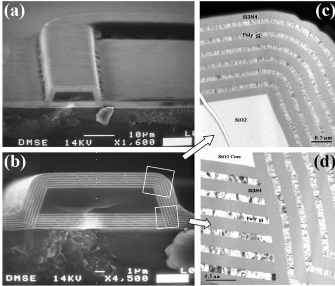
Fig. 4. SEM and TEM images of Bragg cladding waveguide. (left) SEM images of PBG waveguide. (a)  $1600\times$ . (b)  $4500\times$ . (right) TEM images for top corner and bottom corner. (c)  $5000\times$ . (d)  $8000\times$ .
