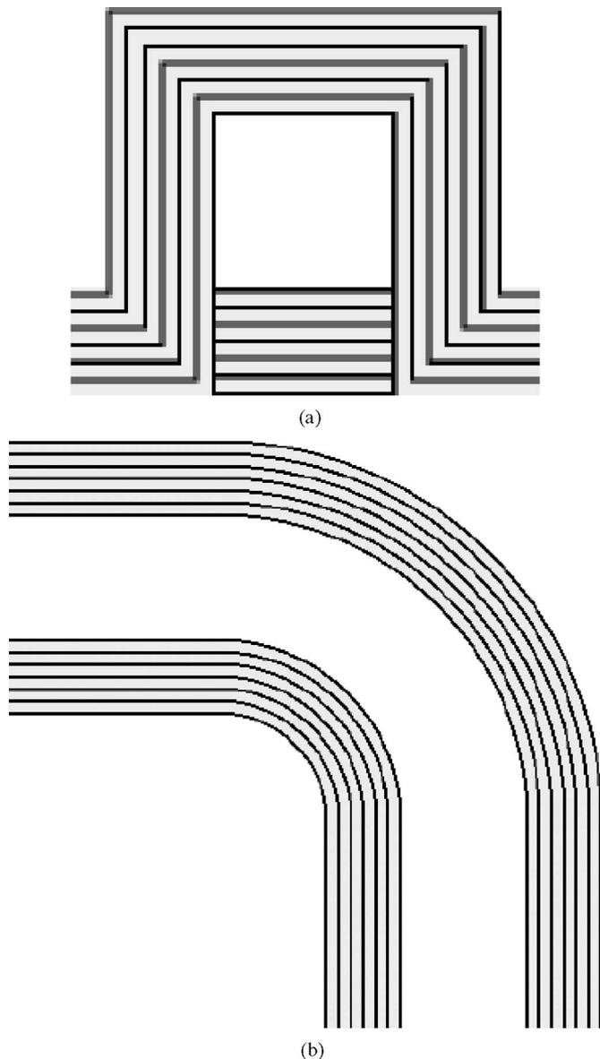
Fig. 1. (a) Bragg cladding waveguide schematic: Bragg cladding layers surrounds low index core. Bragg layers consist of polysilicon ( $n = 3.5$ ) and silicon nitride  $n = 2.0$ ). (b) Cutaway view of 3-D bend, which locally has an on-chip Bragg cladding channel waveguide cross section everywhere.
