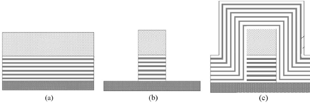
Fig. 3. Waveguide fabrication schematic. All steps are done by conventional CMOS process. (a) Deposit thick oxide (LTO) on Bragg under-cladding layers and densify it. (b) Lithography and dry etch patterning. (c) Deposit top cladding layers using LPCVD process (not to scale).
