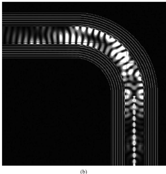
Fig. 2. (a) Transmission spectrum around a  $90^\circ$  bend for a Bragg cladding channel waveguide structure with an inner radius of  $8a$ . (b) Distribution of electric field power for light being guided around a  $90^\circ$  bend. The source is the narrow array of bulges in the lower right. Virtually no power is observed to leak from the waveguide suggesting that most losses about the bend are a result of reflection.
