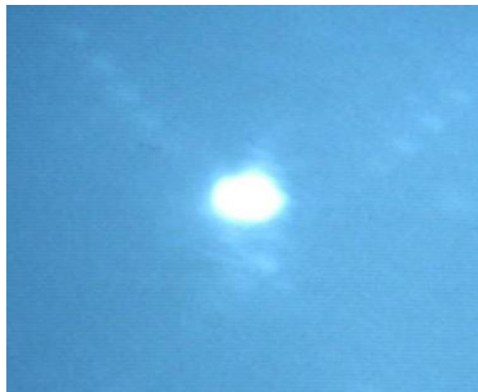
Fig. 3. (a) The TEM image of the fabricated Bragg clad channel waveguide. The smooth interface and good conformal step coverage by LPCVD method are clearly seen. (b) The guided spot from the Bragg clad channel waveguide with dimension 4\mu\text{m} \times 4\mu\text{m} , which demonstrated the guidance in the low index \text{SiO}_2 materials by PBG guiding mechanism.
